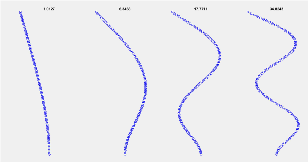
Figure 25. Mode shape as abeam (rad/sec).
